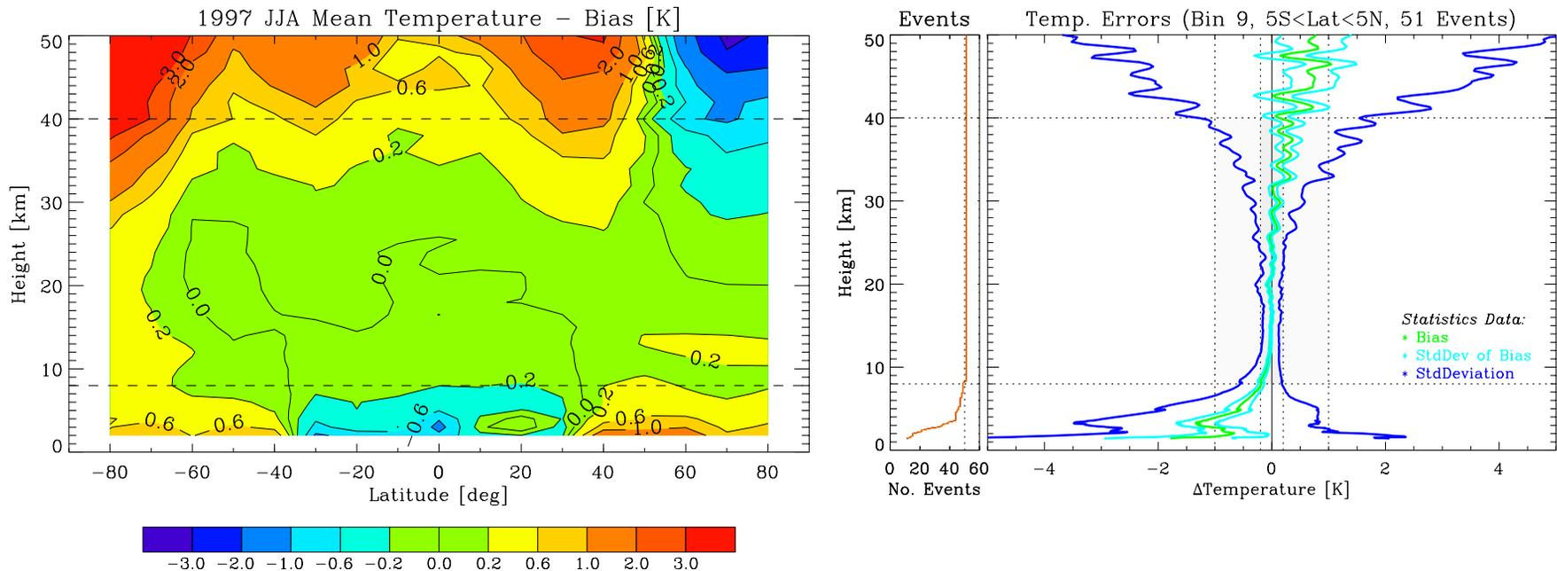
Illustration of retrieval performance using GNSS-LEO occultation data (realistic end-to-end simulations; *left*: lat-height slice of temperature errors of ~50 profile mean, *right*: vertical error structure at equator)
